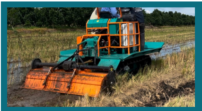
Farming tool lifting system with 1-way hydraulic cylinder, helping farm tools self-lift when encountering obstacles
