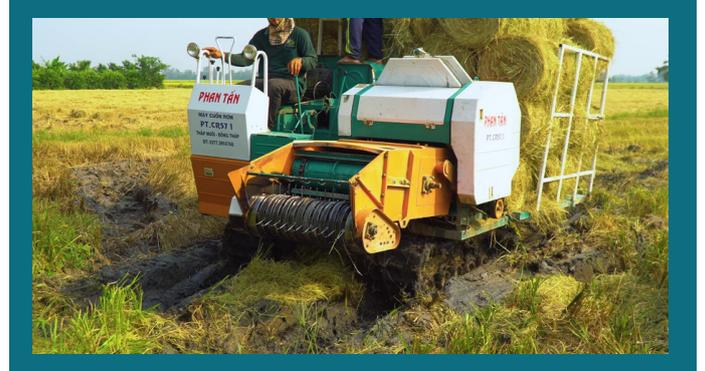
Easy working on the dry, wet and muddy field with the self-propelled rubber tracks.
