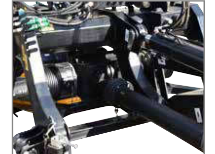
The gear box: Designed for driving powers of up to 400 hp.
