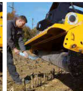
Easy adjustment of the swivelling support roller, even without an assistant.
