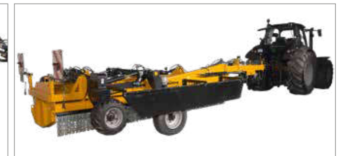
Extended protection against stone projection: Maximum safety for your tractor and the surroundings (optional).
