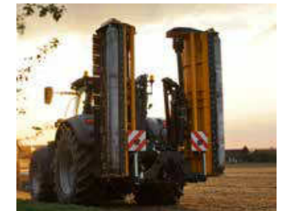
Clever folding: Minimal equipment height due to the parallelogram-type suspension of the two mulcher housings.
