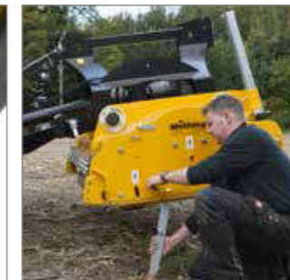
Easy adjustment of the swivelling support roller, even without an assistant.
