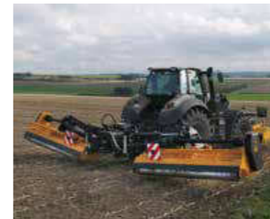
Folds up fast thanks to the freewheels in the final drives.
