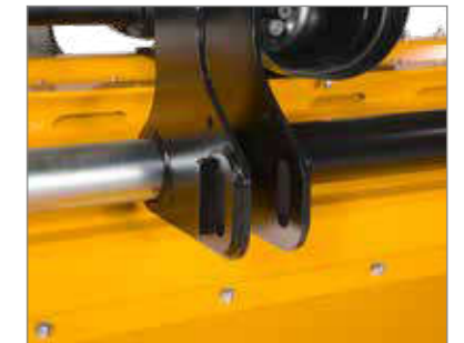
Elongated holes in Cat.3N on the upper and lower link mounting points ensure excellent ground following in combination with the swivelling support roller.
