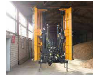
A clever design allows the MU-PRO/F mulcher to be folded up for space-saving storage.
