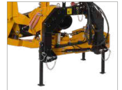
Automatically locking, mechanical transport safety device for quick departure readiness.
