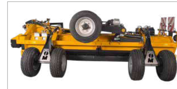
Twin-tyred field chassis for low-impact weight distribution and precise depth guidance.
