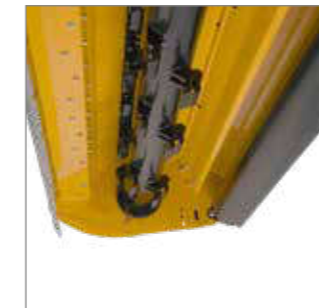
The integrated material guiding flap ensures blockage-free discharge.
