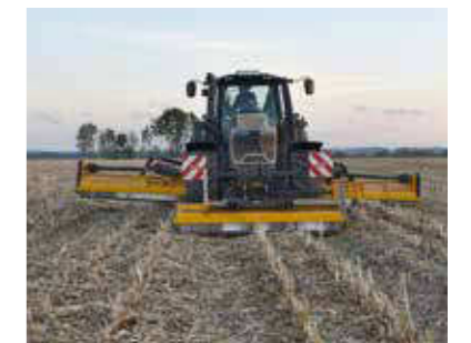
The mulcher housings can also be lifted individually (optional).
