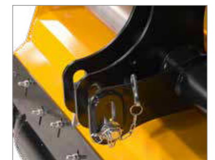
Elongated holes on the upper and lower link mounting points ensure excellent ground following in combination with the swivelling support roller.
