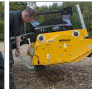
Easy adjustment of the swivelling support roller, even without an assistant.
