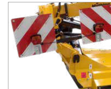
Warning signs with lighting equipment and lighting beam with sturdy mounting wwwand without moving parts
