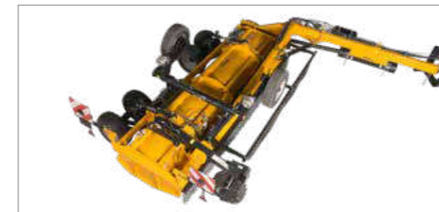
Road transport: Quickly reconfigured from the driver's seat and manually secured.
