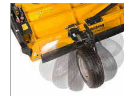
4 low-impact support wheels for vertical adjustment of the Farmer unit for rear mounting. 180° swivelling for high manoeuvrability at the headland.
