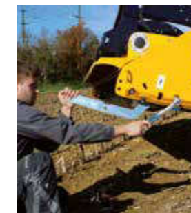
Easy adjustment of the swivelling support roller, even without an assistant.
