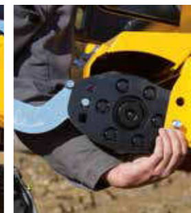
Easy adjustment of the swivelling support roller, even without an assistant.
