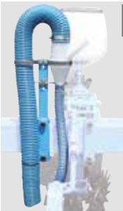
The cyclones assembled opposite each metering unit allowing the fertilizer drop by gravity and thus limiting the dust forming due to the pulsed air.
