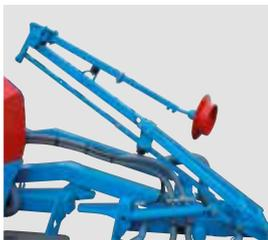
The pivoting row markers enable a compact folding for a minimum transport dimension
