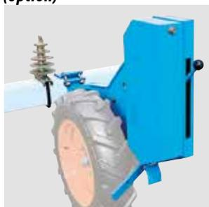
For even easier access, a rear seed spacing gearbox with integrated wheel unit is also available. This seed spacing gearbox with interchangeable sprockets gives and even more precise adjustment for seed population.
