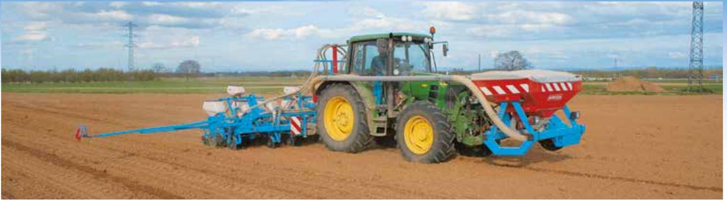
The front-mounted MONOSEM hoppers have been specially designed for fertilizer applications. The sturdy frame with integrated cradle and the 100 % stainless steel distribution unit indicate the care that is applied to manufacture. The turbofan can be driven by PTO or hydraulic motor. The front mounted hopper is multi-purpose and can be mounted on a MONOSEM cultivator for fertilizing whilst cultivating.
