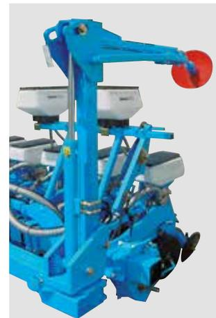
The pivoting row markers enable a compact folding for a minimum transport dimension
