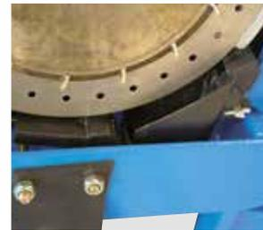
The seed monitor sensors are placed under the metering boxes. A beam of light enables the control of the seed passage, even the smallest seeds.
