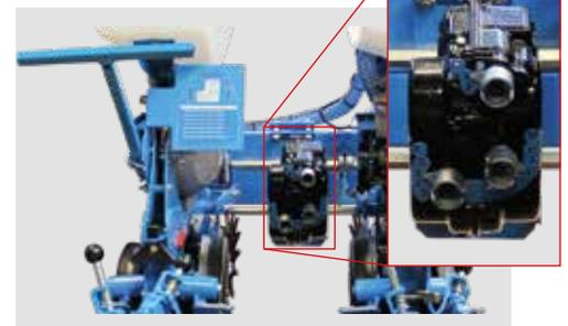
Available on option (except on Extend, Monoblock2 and TFC rigid frames), the EasyGear seed spacing gearbox allows an easy adjustment of the seed population. Thanks to its 3 levers, it offers 18 ratios perfectly levelled and is maintenance free.
