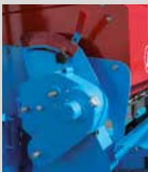
Easily accessible on the side of the planter, the FertiDrive<sup>VM</sup> variable speed transmission allows very quick and easy adjusting of the quantity of fertilizer per hectare required. This transmission is also equipped with a disengaging mechanism, used to stop the fertilizer intake where it is not necessary.
