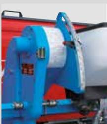
The Microsem has a MicroDrive<sup>VM</sup> variable speed drive easily accessible on the side of the planter for a quick and easy adjusting of the required dose. This transmission is also equipped with a disengaging mechanism, used to stop the Microsem intake where it is not necessary.
