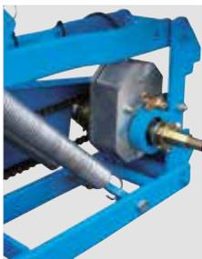
Electromagnetic clutch on NG Plus 4 metering unit
