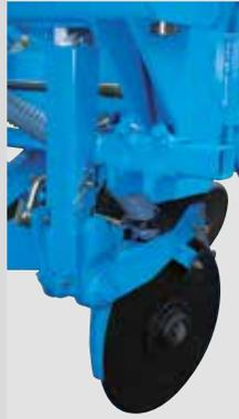
On the Extend planter, a Double function turbofan (Df) ensures an efficient vacuum suction of the seeds and also to pulse the fertilizer on the outer rows to efficiently distribute at 45 or at 80 cm inter row spacings. On the pulsed rows, a stainless steel cyclone is integrated on each fertilizer disc.
