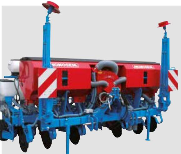
The « High capacity » hoppers in sheet metal on Monoblock, single or double telescopic frames have a capacity of 980 L.
