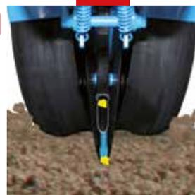
The curved seed chute tube has been specially designed to accompany the seeds gently into the ground and with a perfect accuracy.
