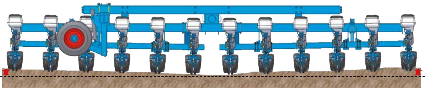
On the wide configuration frames, a correct following of the ground contours is essential. This is why each frame making up a coupled frame is independent and has articulations allowing for a perfect following of the ground contours.
