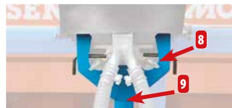
The capacity of the Microsem hoppers is 20L. 40-litre hoppers are also available on option (Assembly according to frame). The trapdoors (8) and the chute (9) allow for a simple and quick emptying of remaining product.
