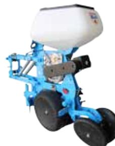
NG Plus 4 metering units can be equipped with electric drive of the distribution. Each distribution is driven by an electric motor thanks to a notched belt. Located on the planter, the ECU module allows the user to manage the seed population from the tractor cab thanks to the ISOBUS TOUCH Mini or TOUCH terminal. This system is compatible with the automatic row cut-off system by GPS (TC-SC function).
