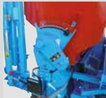
Easily accessible on the side of the planter, the FertiDrive™ variable speed transmission allows very quick and easy adjusting of the quantity of fertilizer per hectare required. This transmission is also equipped with a disengaging mechanism, used to stop the fertilizer intake where it is not necessary.
