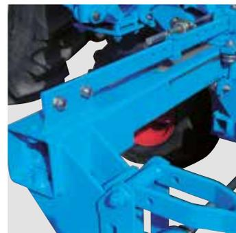
The hydraulic telescopic bars ensure the lateral movement of the metering units in order to change inter row spacings.
