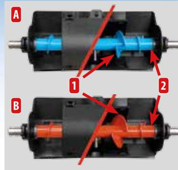
The « Standard » augers (A) in blue are for fertilizer metering from 80 to 350 kg/ha for an inter row spacing at 75 cm and from 120 to 525 kg/ha for an inter row spacing of 50 cm.
