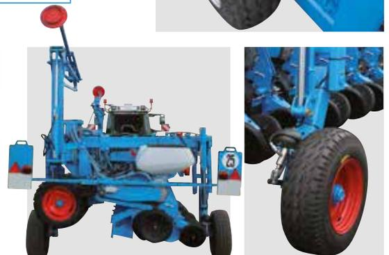
For easier transport, a lengthwise transport carriage is available on option. This transport carriage is equipped on option with a hydraulic or air brake system.
