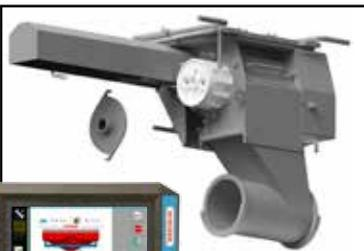
On the Standard and DUO front-mounted hoppers with electric drive, the quantity of fertilizer is managed from the tractor cab via the ECU F800E and the ISOBUS touch terminal (TOUCH or TOUCH Mini). The front fertilizers with electric drive have an easily-removed and without tools dosing wheel and metering anticipation function.
