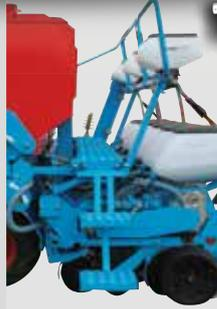
On the Extend planters with fertilizers, a platform, delivered as standard equipment, enables an easy access to the fertilizer hopper. The platform and the step thus enable a safe access to the hopper during filling operations.
