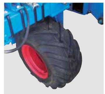
The wide wheels with large diameter ensure a regular and constant drive of the seed discs. The rapid adjustment of the width of the drive wheels means a rapid adjustment to the different tractor treads.
