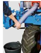
The « High Capacity » fertilizer hoppers are equipped with a trapdoor on each side with a hose enabling a rapid and easy emptying of the hoppers.
