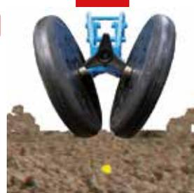
The rear press wheel unit, made up of 2 V-wheels, closes the furrow around the seed for optimal seed germination.
