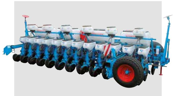
12-row rigid Double bar planter (45 cm inter row spacing) with lengthwise transport carriage
