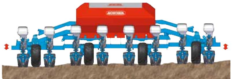
The TFC and TFC2 frames have independent wings with wheel units. This characteristic allows for a perfect following of the ground. At the field ends or to finish off a field, it is also possible to lift one or other of the wings (or the 2) thus automatically stopping the metering.
