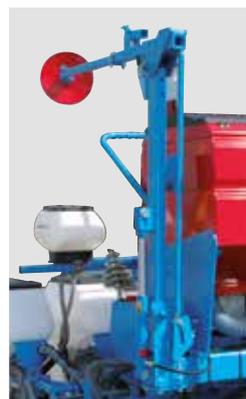
The folding row markers allow marking at the wheel or in the centre but take up little space when in transport. They are also equipped with a safety system and a mechanical locking system for the transport.
