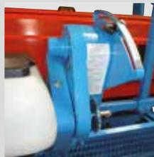
The Microsem has a MicroDrive™ variable speed drive easily accessible on the side of the planter for a quick and easy adjusting of the required dose. This transmission is also equipped with a disengaging mechanism, used to stop the Microsem intake where it is not necessary.
