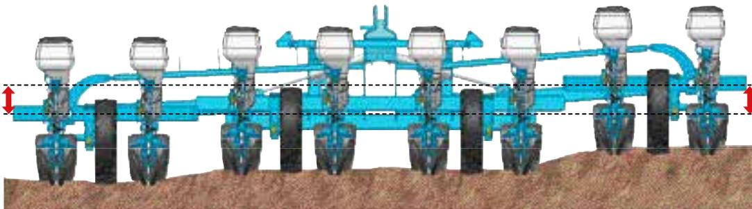
The floating Double bar folding frame has independent wings with wheel units. This characteristic allows for a perfect following of the ground. At the field ends or to finish off a field, it is also possible to lift one or other of the wings (or the 2) thus automatically stopping the metering.
