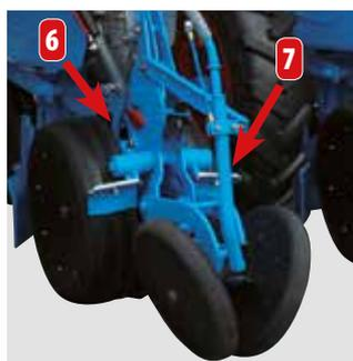
The Insecticide Microsem chute (6) is placed between the 2 discs for product supply in the planting line. The Helicide Microsem chute (7) is adjustable for a product supply on the planting line before or after the passage of the press wheels.
