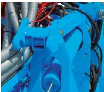
The wings are automatically locked in transport position. The locking is made from the tractor cab.
