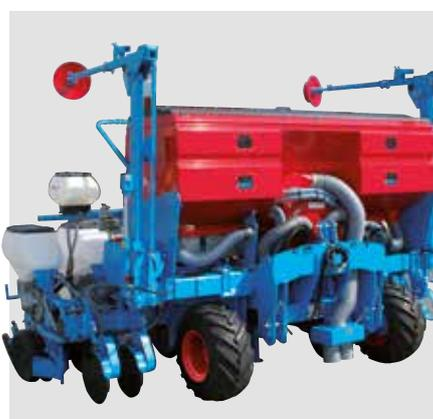
The « High Capacity » hoppers in sheet metal on the single and double telescopic Monoblock2 Comfort frames have a capacity of 680 L or 1030 L. On the Extend frames, the capacity is 1020 L. This capacity is 1500 L on the TFC folding frames.
