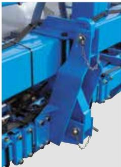
The fixing system of the planters on to the coupling bar allows each unit to follow the ground contours.
