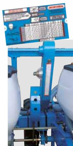
Adjustment of the microgranulators is made using a gearbox with 18 ratios. If needed, other sprockets are available and also a rapid declutching system.
