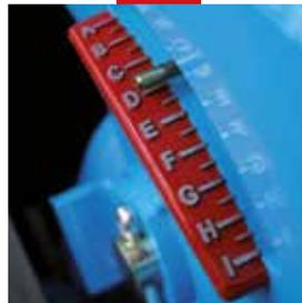
The depth adjustment index is visible straight away from the rear. It is weather-proof.
