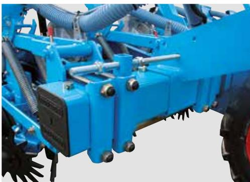
The stop parts on the telescoping system enable an adjustment perfectly suited to the required inter row spacing and folding that is suited to the equipment of the planter.
