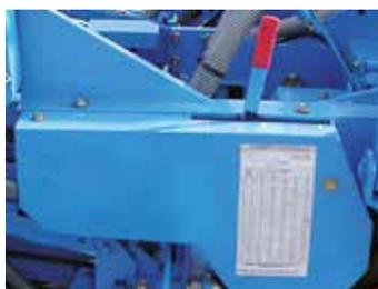
The drive of the metering unit is ensured by a reinforced transmission. The seed spacing gearbox is situated on the extreme left side of the planter for easy access and a rapid changing of the sprockets. The 20 settings with interchangeable sprockets offer a wide choice of seed populations.
