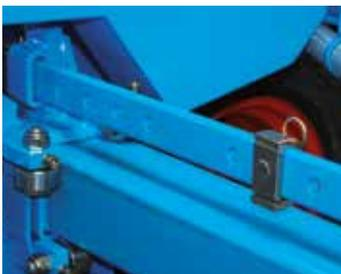
The adjustment of the inter row of the NG Plus 4 Extend planter is very simple. You just have to position the stop parts on the adjustment bar on the required spacings and then lengthen or shorten the hydraulic cylinders on the telescopic bars in order to obtain the desired spacing.
