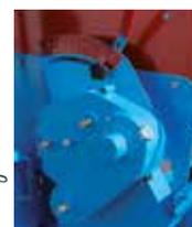
The fertilizers on the Monoblock2 Comfort, Extend and TFC frames are equipped with a variable speed transmission for simple and precise adjustment of the quantity of fertilizer to be distributed.
