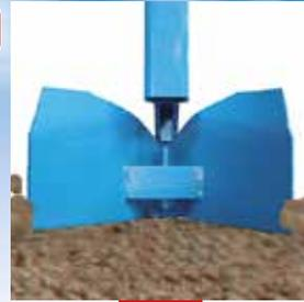
The clod removers or the trash wheels clean the way for the future planting line pushing out clods, stones or trash.
