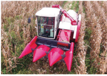
Special three rows semi-feeding corn header with row distance 600mm/750mm
