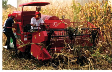
Special three rows semi-feeding corn header with row distance 600mm/750mm
