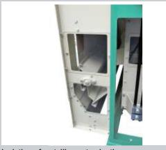
**Isolation of metallic contamination**An optional magnet in the vertical sifter removes metallic objects out of the main product.
