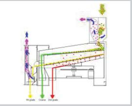
**Optimal cleaning**With combined inlet and outlet aspiration the GrainPlus meet the highest requirements by very dust laden products.
