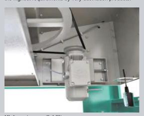
**High system availability**Safety equipment such as the oscillation monitor on the screen box provide protection against malfunctions.
