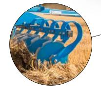
**Low-wear, serrated concave discs** With a diameter of 510 mm
