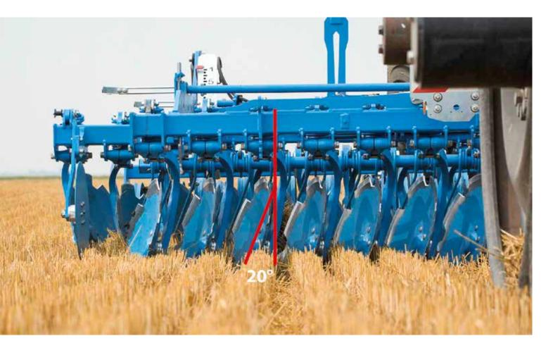
The concave discs of the **Rubin 10** are attached individually to a surface hardened stalk. Its special shape provides maximum space between the discs. The optimised clearances between the discs enable the **Rubin 10** to operates without clogging, even under very damp and sticky conditions.
