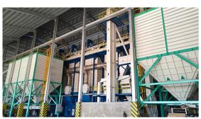
1 set 5 units Grainpro Grain Dryer 30 Tons with Cyclonic Husk Furnace CHF-2000 (Guimba, Nueva Ecija)
