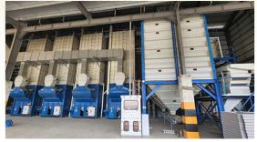
2 sets 8 units Grainpro Grain Dryer 30 Tons with Cyclonic Husk Furnace CHF-3000 (Muñoz, Nueva Ecija)
