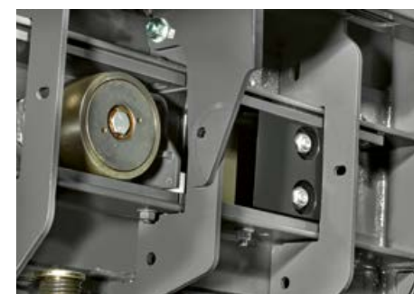
The rotating knives can be mounted in two positions for use in straw / maize straw or in hay / silage.
