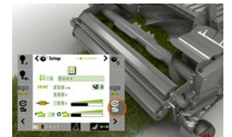
The POWER FEEDING SYSTEM is easily reversed from the driver's cab.
