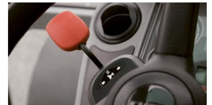
Operate the REVERSHIFT clutchless reverser with your fingertips.
