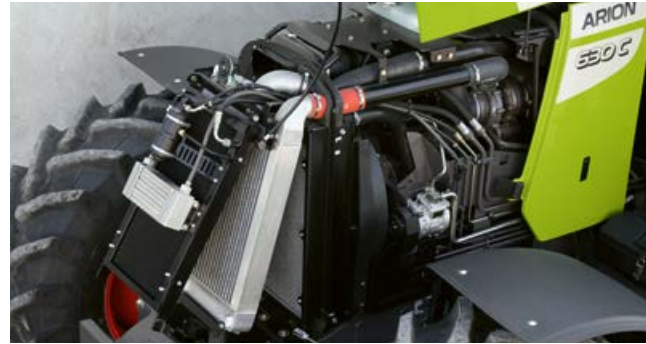
The radiator can be quickly tilted to one side for cleaning.
