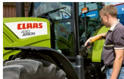
The large fuel tank on the ARION 400 minimises tank filling time and therefore reduces downtime. Its 175 litre capacity allows long, productive days.
