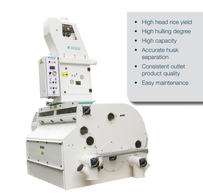
Designed to be powerful and reliable - TopHusk, the new compact huller and hull separator from Buhler is a perfect fit in your modern rice mill. TopHusk is well equipped to give your milling process a head start.
